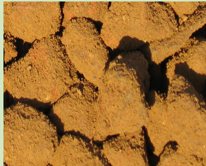
Figure 11. Davis Soil, a non-loadbearing soil (i.e. not a structural soil) with high infiltration rate and high potential for water storage.
