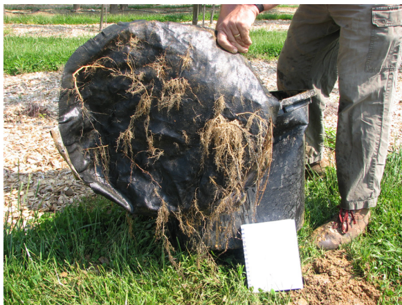
Figure 19. Ash roots penetrating geotextile after compacted subsoil has been washed away. Roots increased infiltration by a factor of 27. Photo by Susan Day.
