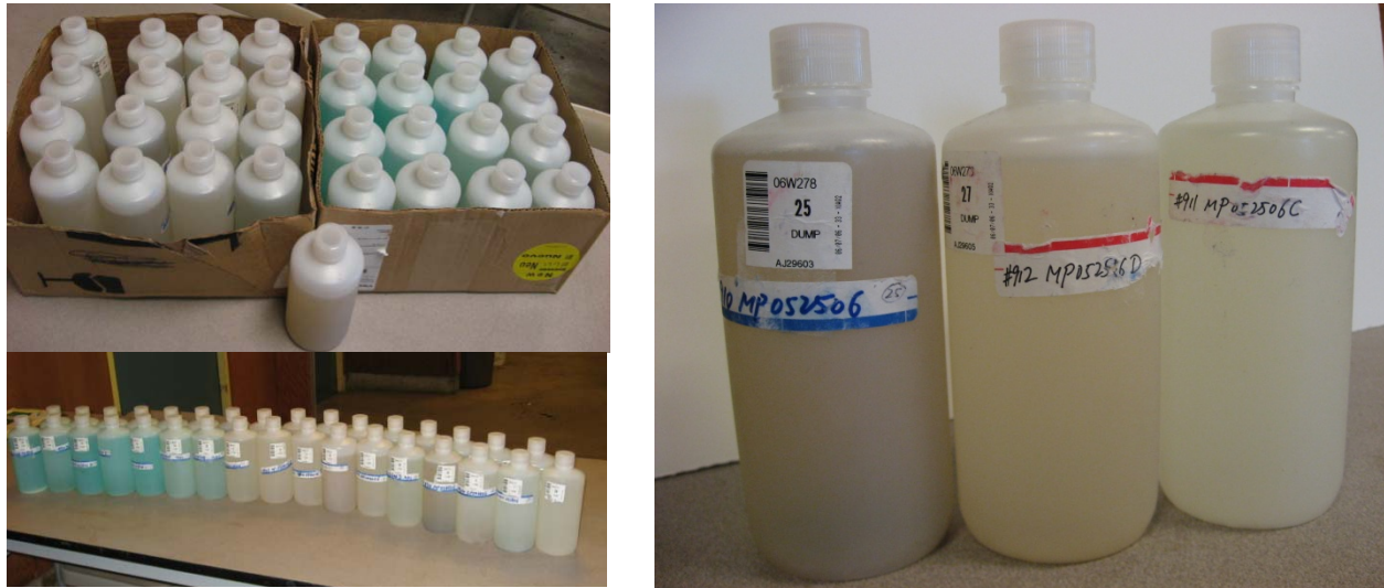
Figure 10: Water quality testing, water samples from each test were stored in a 500 ml water bottle for water quality analysis. The green-blue water color in the left image is the synthetic runoff that was mixed with natural runoff and fertilizer. The image in the right shows the runoff before (left) and after passing through the soil column (middle and left).
