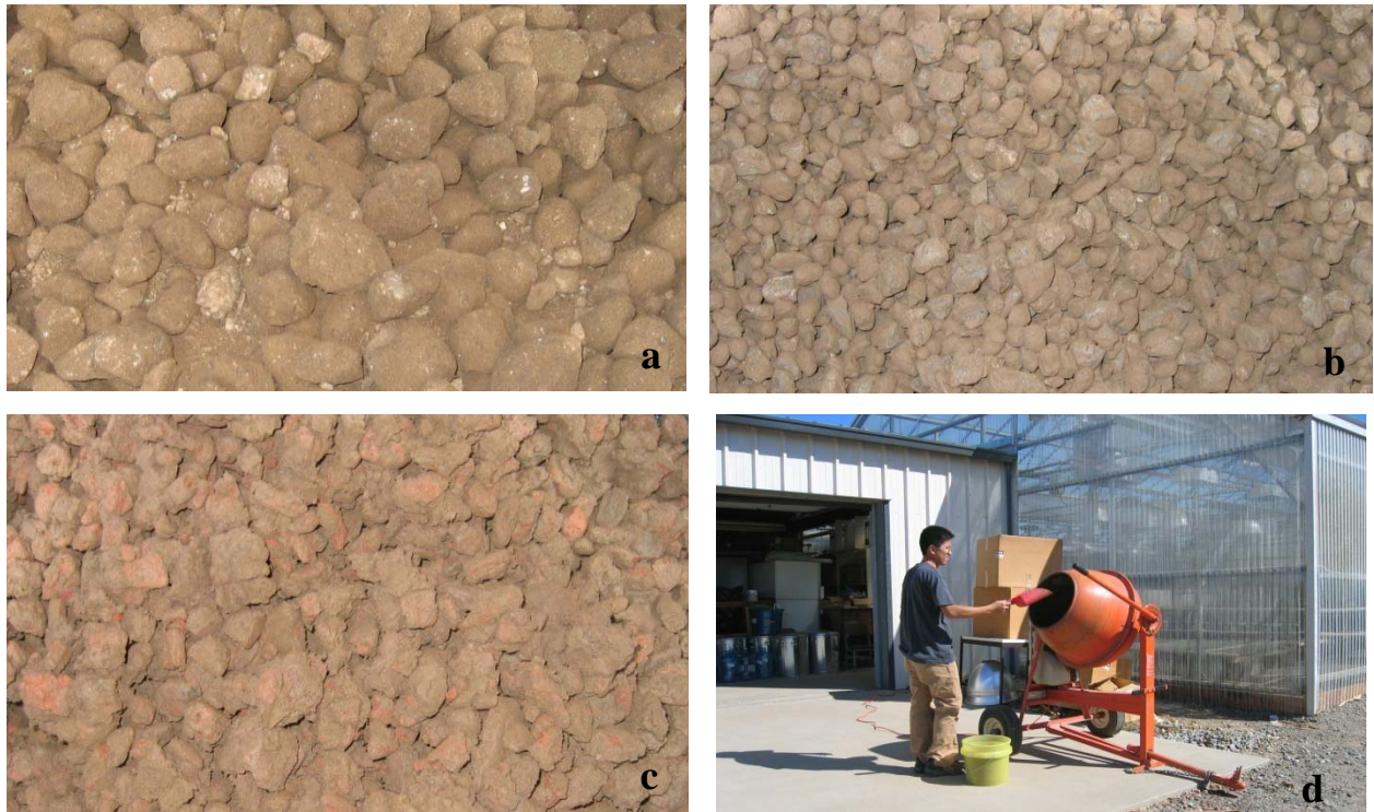
Figure 1. Engineered soils (a) CU soil. (b) CS soil. (c) DS soil. (d) Using soil mixer to make DS soil.
