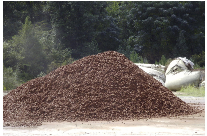
Fig. 1.8 From upper left, clockwise: uniformly-graded crushed stone of 3/4” - 1 1/2” diameter, pile and close-up; CU-Structural Soil™ after mixing; clay loam.
