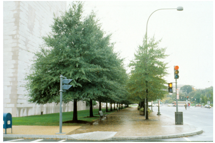
Fig.1.6 This photograph shows the effect of soil volume on tree growth. Both rows of willow oaks were planted at the same time on Pennsylvania Avenue, Washington, D.C. The trees on the right are in tree pits, and those on the left are in an open grassed area.
